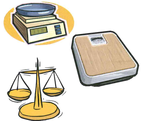
Figure 1-18: Drawing of scales and a balance— instruments used to measure weight. Weight depends on the gravitational acceleration experienced on the surface of a planet.
